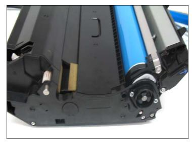
2. Turn the drum unit clockwise to commence disassembly on the right side of the OPC drum.
