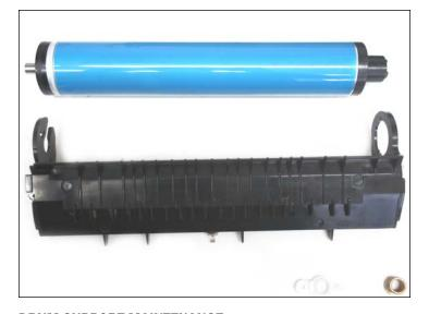
**DRUM SUPPORT MAINTENANCE** 16. Clean and vacuum the drum unit thoroughly. Assemble following the disassembly steps in reverse.
