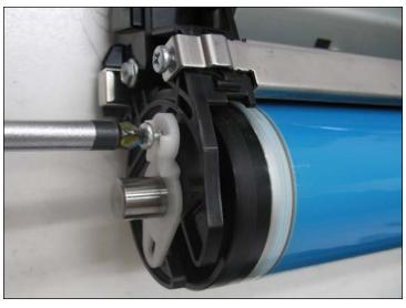
10. Unscrew the drum axle support as shown.
