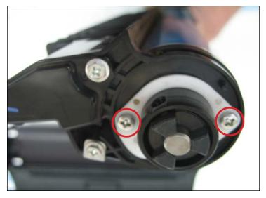
13. On the right side of the OPC drum, unscrew and remove the plastic bearing (shown).
