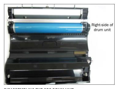
**DISASSEMBLING THE OPC DRUM UNIT** 1. Arrange the OPC drum unit as shown.
