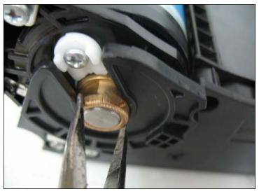
6. Using a pair of needle-nose pliers, grip the copper bearing (shown) turning it clockwise to release the OPC drum.
